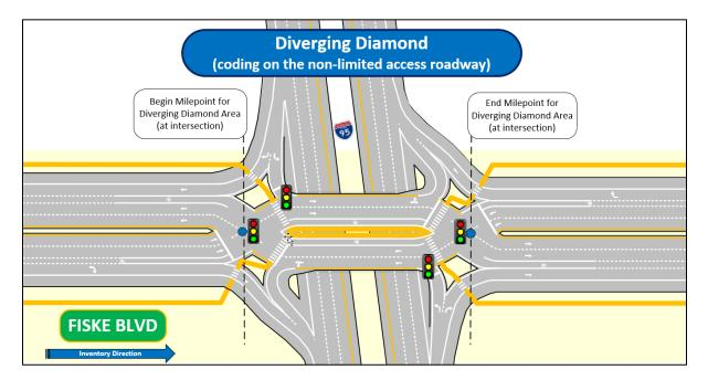
In this example, the inventory direction is from west to east. The BMP for DDIXOVR is coded at the center of the intersection on Fiske Blvd on the west side of the crossover area. The EMP for DDIXOVR is coded at the center of the intersection on the east side of the crossover area.
